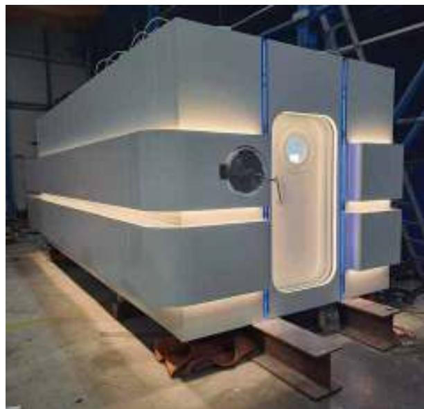
This construction contributes to the controlled high-pressure environment necessary for effective HBOT. The robust materials and engineering guarantee the chamber's ability to maintain specific atmospheric conditions while accommodating multiple patients.
